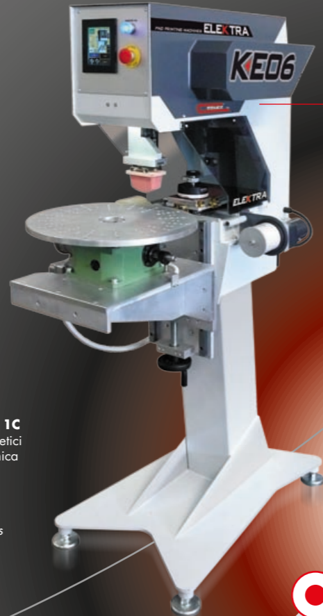
KE-06 Elektra 1C with hermetic ink cups and 90 mm diam. ceramic rings
